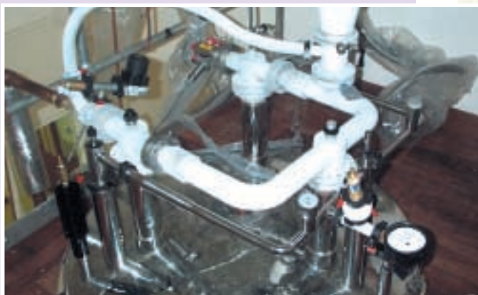
Top view of the magnet detailing the 2.3K manifold hardware.
